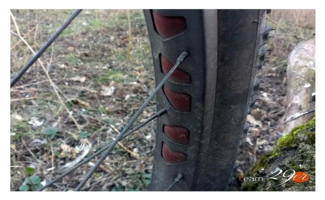
Heavily perforated rims are very difficult to convert to tubeless system, and so for the "ease" of life, Michael Travers offers a classic inner tube. But do not count on the low weight, because here we have two thick and heavy rubbers each weighing 400g! No pain, no gain!
