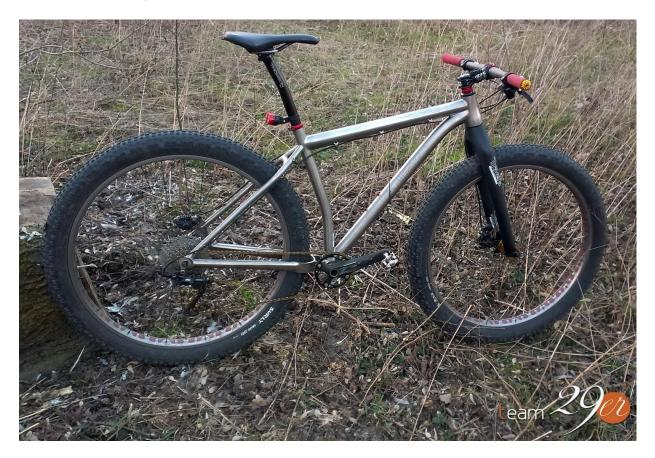
Michael Travers uses the popular and often used alloy Ti3A1-2.5V - the "equivalent" of AL7005. The main tube and the rear triangle have classical cross sections, maybe with the exception of slightly ovalized section of the down tube. Frame-builder did not make an effort to implement some technological and visual wonders. Simplicity, practical sense and minimalism - all are worth appreciating.
